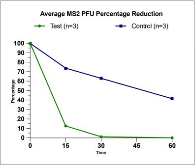
**Figure 5.2.** Average percentage reduction of MS2 PFU/m³ of air over time. Graph is calculated from data points in appendix tables 8.1 and 8.2
