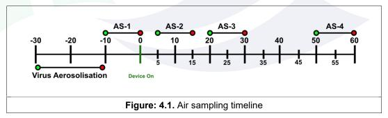
In the active test runs, the air purifier was operated at t = 0 and remained operating for the duration of the test. All air samples collected during testing were transferred to the laboratory for analysis by plaque assay.
