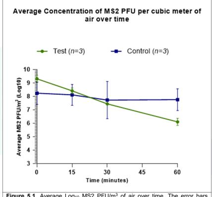
**Figure 5.1.** Average Log<sub>10</sub> MS2 PFU/m<sup>3</sup> of air over time. The error bars represent standard deviation.
