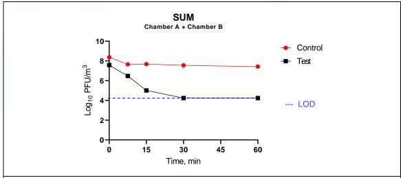
**Figure 5.3.** Sum of the concentration of airborne MS2 determined in test chambers A and B. LOD: limit of detection 4.24 Log<sub>10</sub> PFU/m<sup>3</sup>
