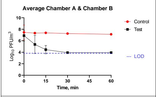
**Figure 5.2.** The average concentration of airborne MS2 determined in test chambers A and B. LOD: limit of detection 3.94 Log<sub>10</sub> PFU/m<sup>3</sup>
