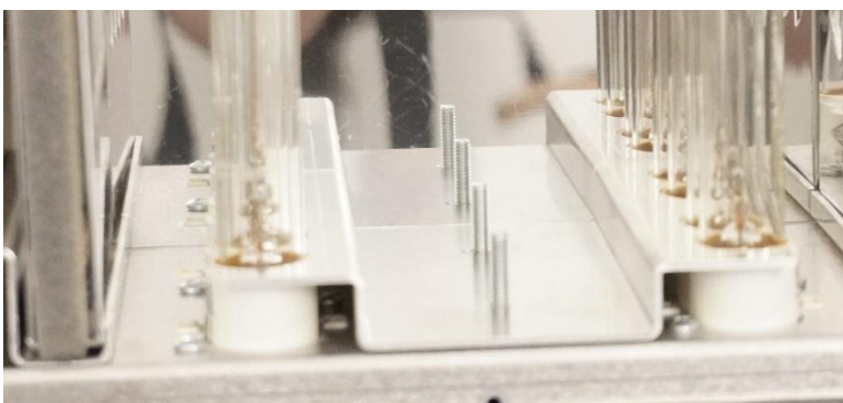
12. Carefully slide bulb retainer over bulbs (top to bottom).
