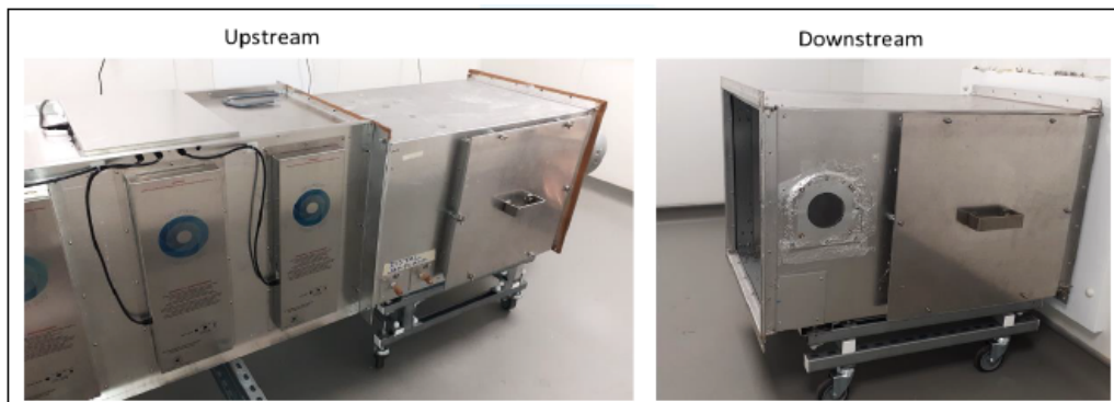
Figure 2.1. Air Sniper Induct 300 unit installed inside the chamber at airmid healthgroup
